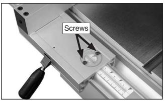
Figure 75. Fence scale window and screws.
